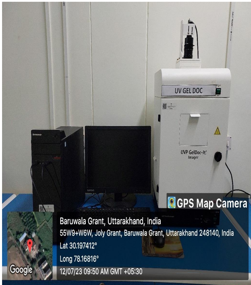
UV-Gel Documentation Unit in Instrumentation Room used to record and analyze the results of gel electrophoresis and membrane blotting experiments
