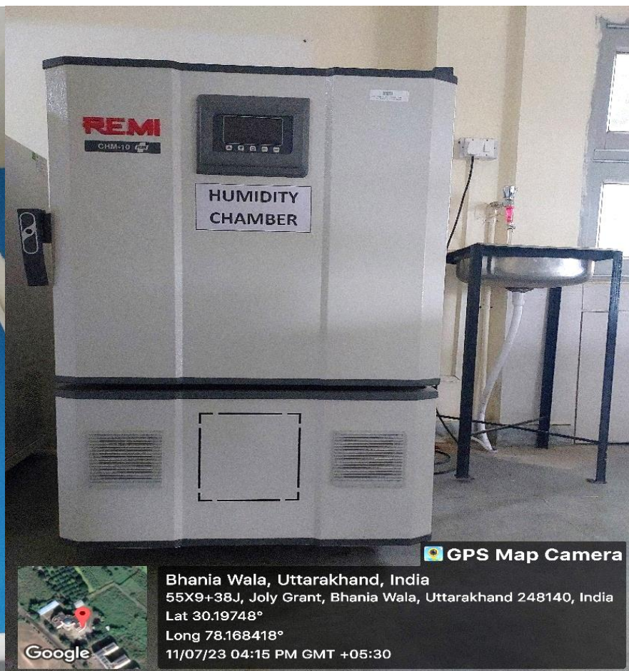
Humidity Chamber in Molecular Biology Lab for incubation of biological samples at controlled humidity
