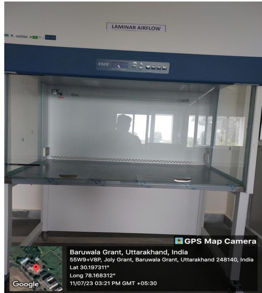
Laminar Air Flow in Advanced Molecular Biology Lab used for performing contamination sensitive processes e.g., plant and animal tissue culture, bacterial culture
